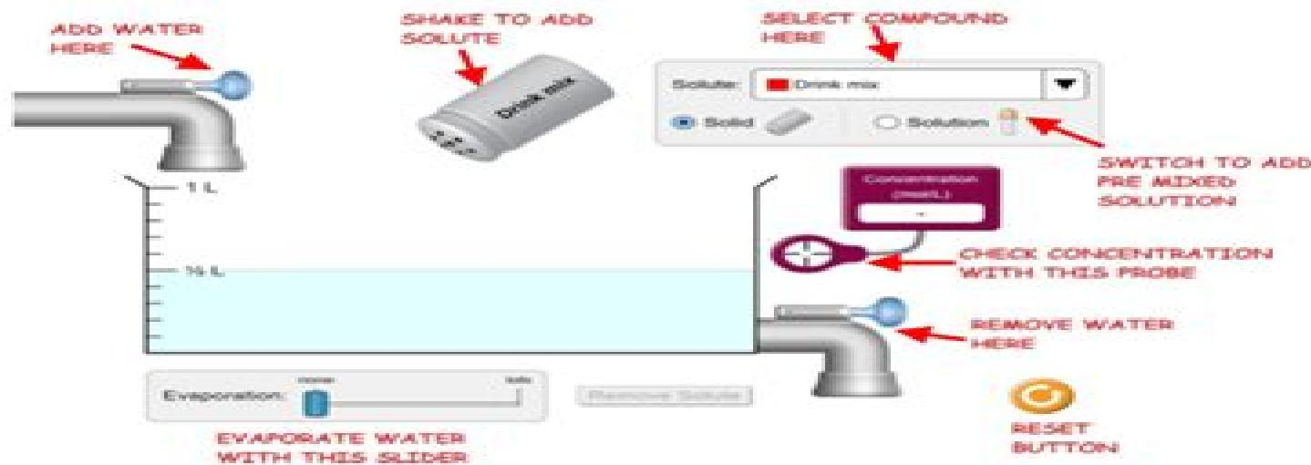
Press Reset. Move the Concentration Probe into the liquid. Then Shake some Drink mix into the water. Continue to add More Solute.
