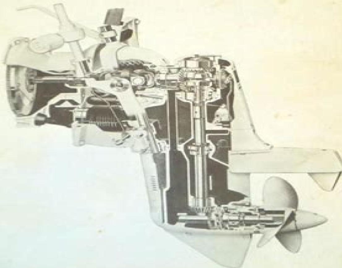
**OUTBOARD DRIVE UNIT MODELS B and C**
