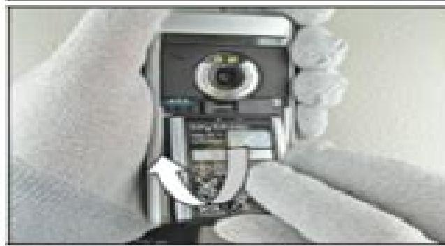
Remove the battery completely from the phone with your fingers.
