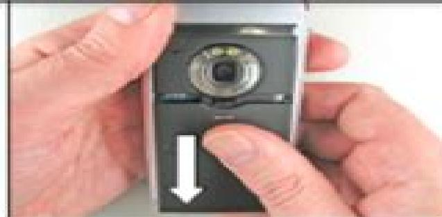
Remove the battery lid completely.
