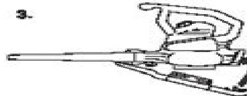
Important: You must install the blower tube before installing the inlet cover because the inlet cover hooks onto the blower tube. The blower will not run unless the bottom inlet cover is locked in place.
