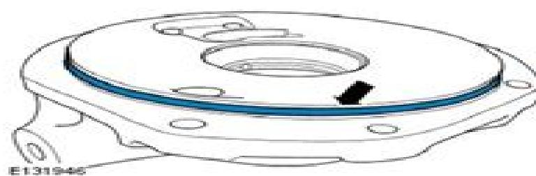
7. Remove the crown wheel assembly.
