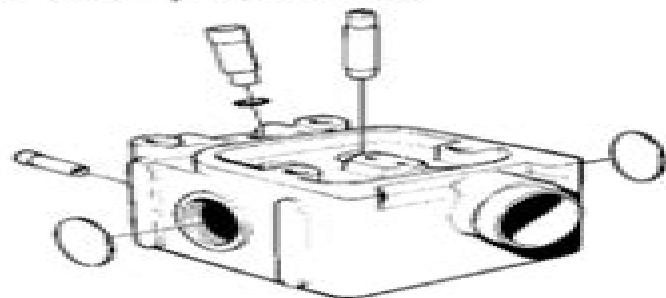
28. Clean all parts. Pay particular attention to coolant passages. In case of doubt, check for leakage by pressure testing. Water pressure 0.3 MPa (3 kg/cm<sup>2</sup> = 43 p.s.i.).
