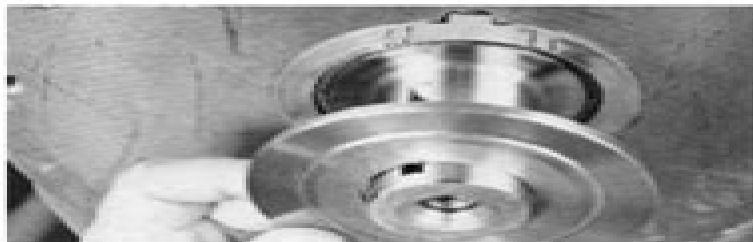
74. Place the engine so that it is resting on the flywheel. Make sure that the inner thrust washer is correctly located. Place the outer thrust washer on the crankshaft with the flat surface towards the main bearing. Fit the distance washer with the flat surface toward the thrust washer.
