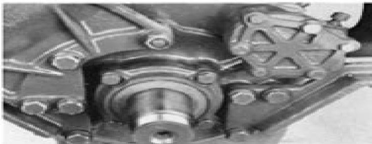
71. Fit the starter motor and the oil pump. NOTE! Put a little oil into the pump before fitting. MD11: Fit the front engine brackets.
