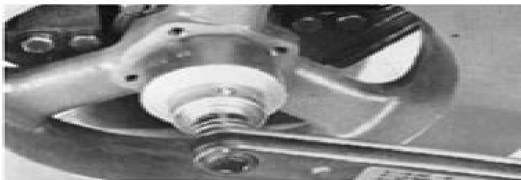
72. Fit the key and the flywheel (the taper must be perfectly clean). Tightening torque: 500 Nm (50 kpm = 369 lb-ft). Lock the nut by bending up the washer.
