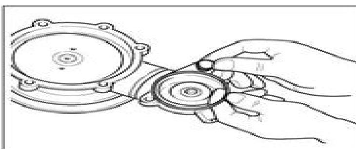
106. Fit the O-ring into the thermostat housing.
