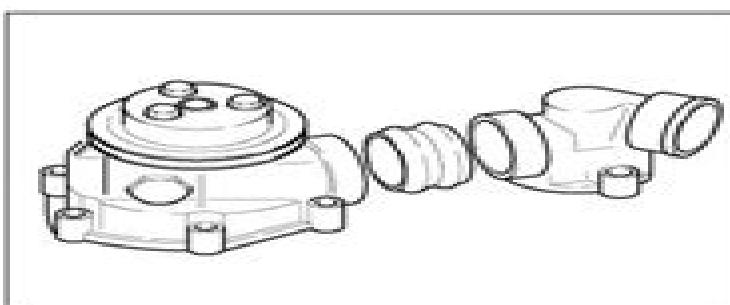
105. Press the intermediate pipe into the thermostat housing and coolant pump.
