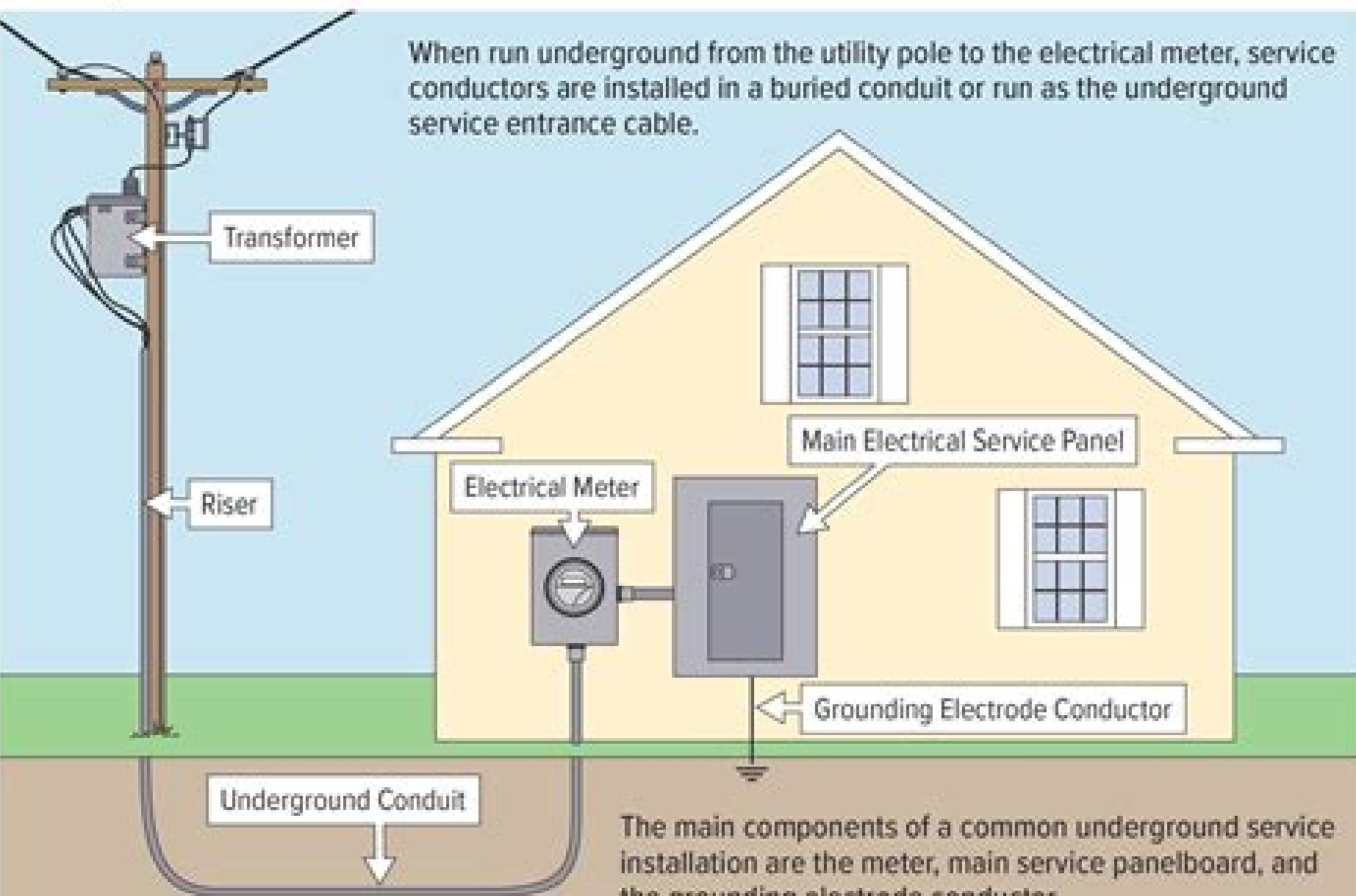
The main components of a common underground service installation are the meter, main service panelboard, and the grounding electrode conductor.
