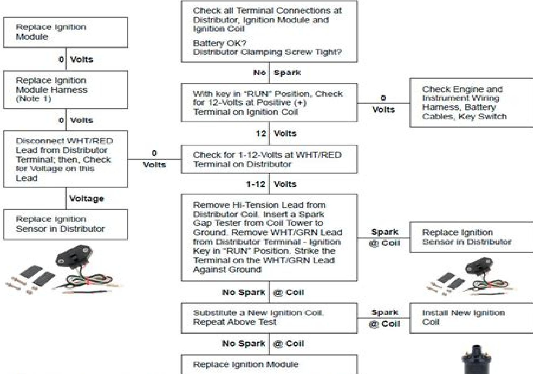
NOTE 1: Early, large ignition modules did not have a replaceable wiring harness.
