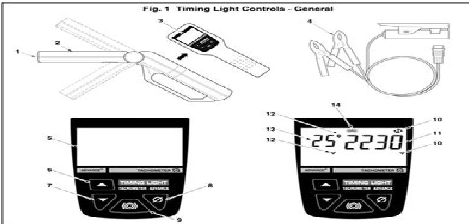
6. **Advance Increment Switch** — Increments through degrees of advance.
