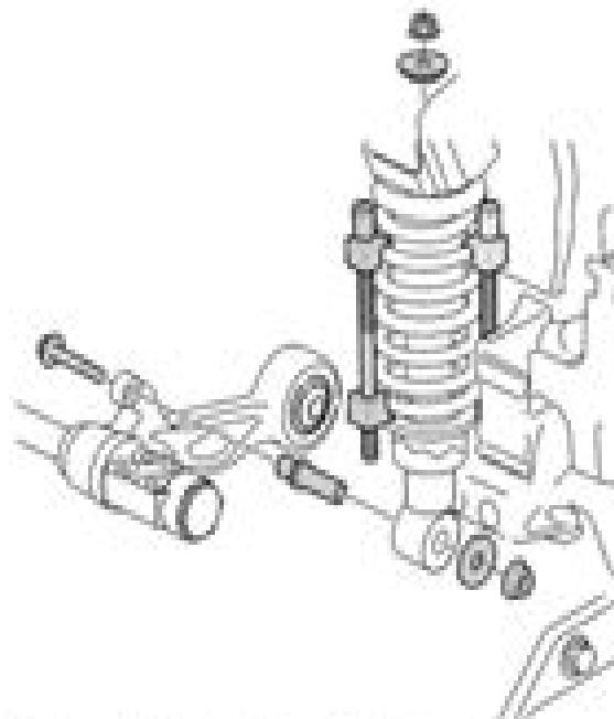
Fit the lifting tool 0000273 and compress the spring.
