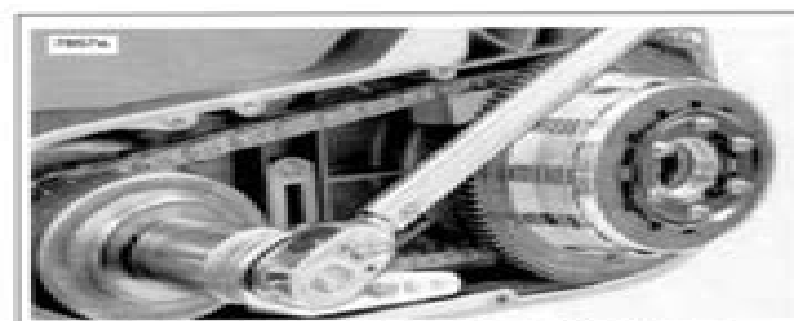
Figure 2. Tightening To 75 ft-lbs (101.7 Nm)
