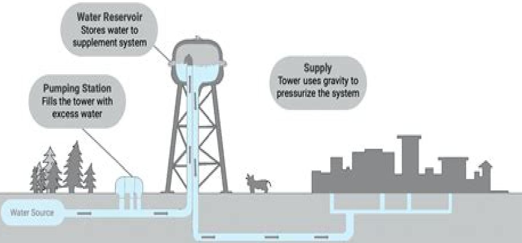
Arboretum tower is part of the UC Davis Domestic Water system for potable water and is sourced from a blend of groundwater (deep aquifers) and surface water (rivers).
