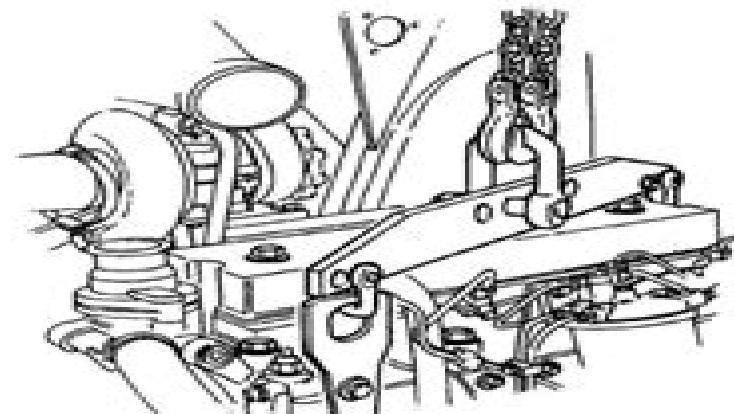
Install the engine lifting bracket (6) using two of the bolts (2) from the air filter bracket. The bracket is part of the machine tool kit.
