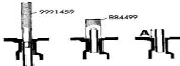
30. Press out the valve guides using drift 9991459. Oil the new guides externally and press them into position with tool 884499. The tool should be pressed right down against the cylinder head. Ream the guides if necessary with broach 9994128.
