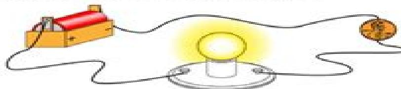
Touch the free ends of the wire to the object you are testing. If the light bulb lights up, the object is made from a conductor. If it does not, the object is made from an insulator.
