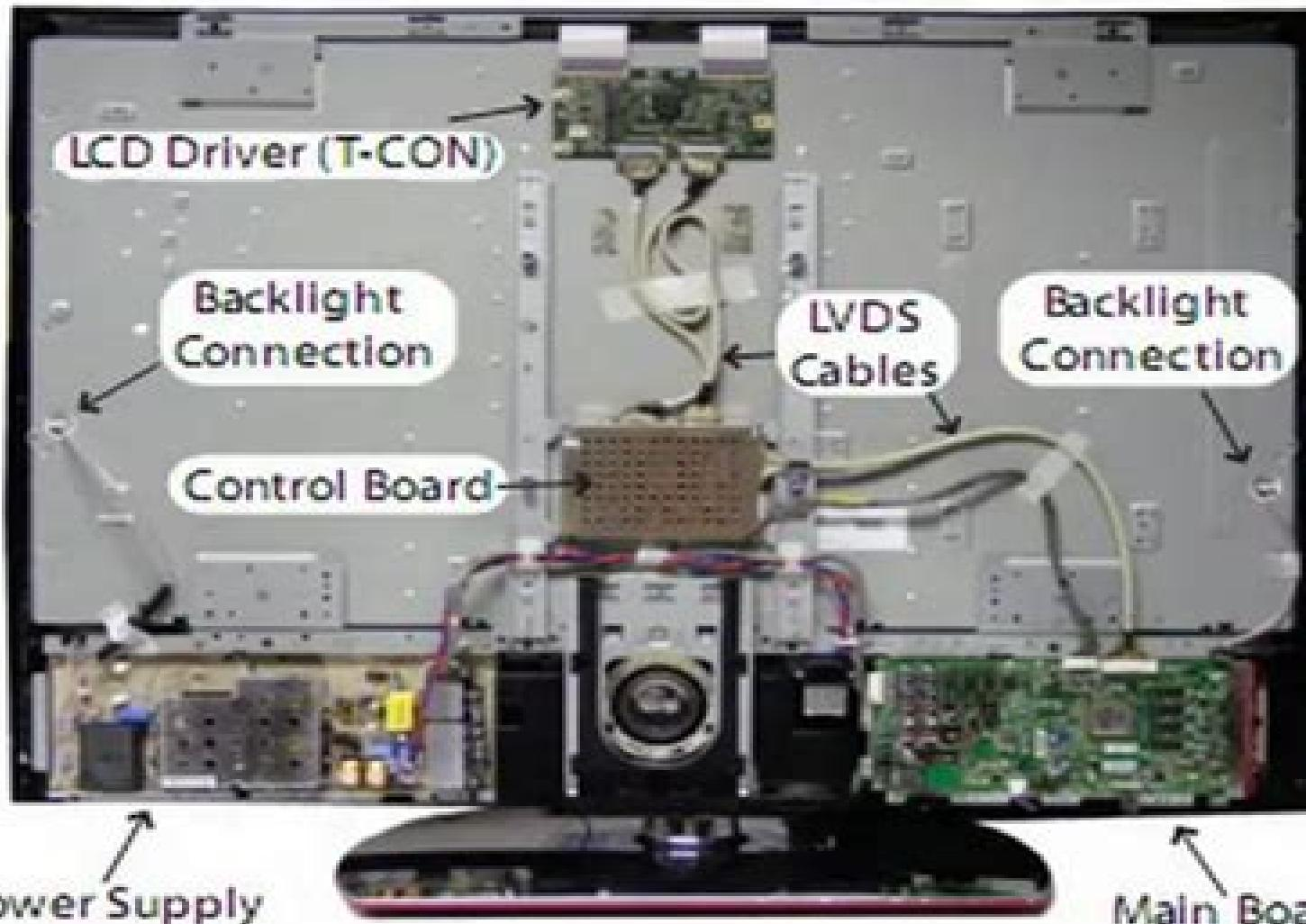
**T-CON - CONTROL BOARD - POWER SUPPLY - MAIN BOARD**
