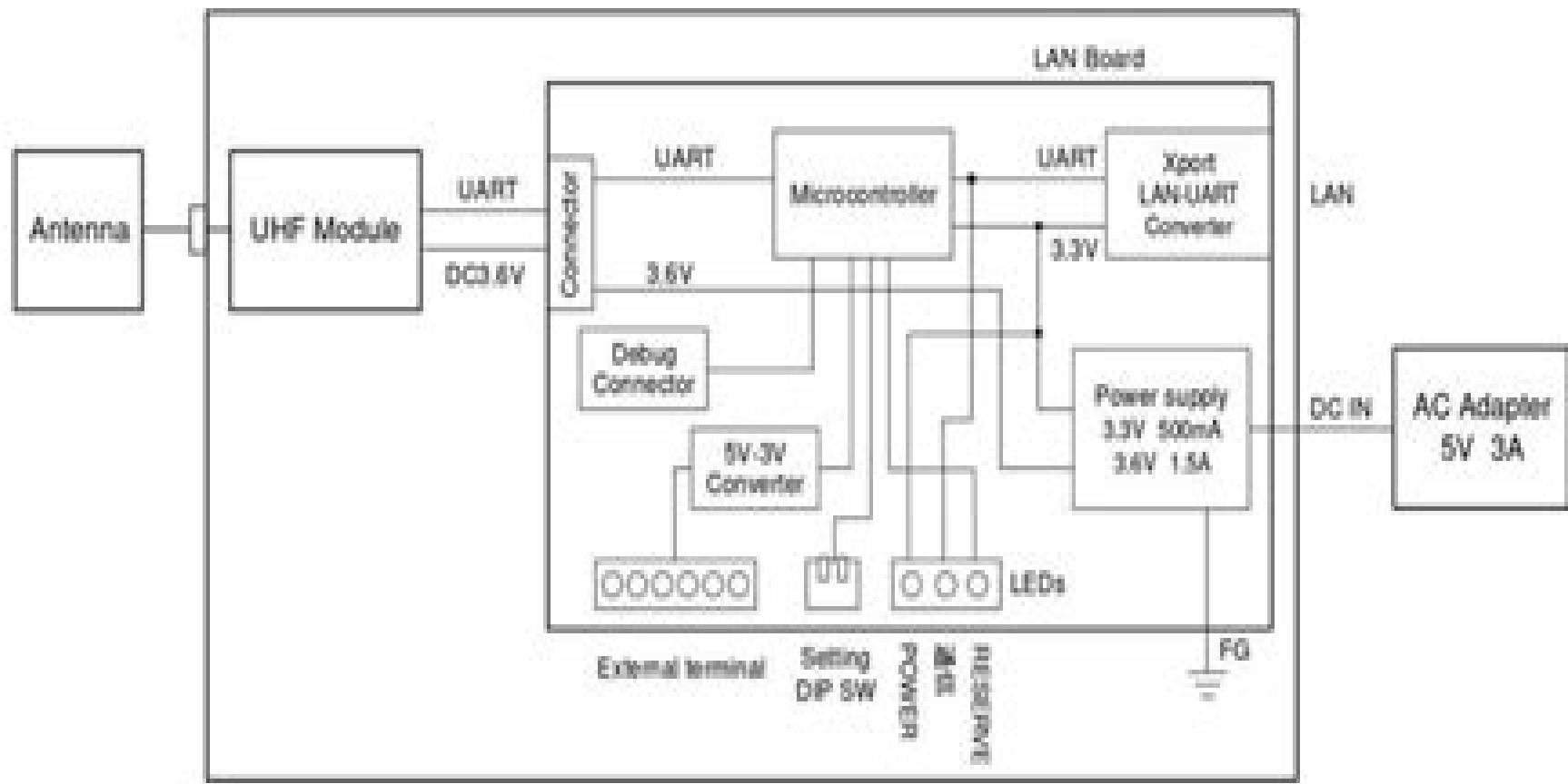
**Figure 2-4 Internal block diagram**
