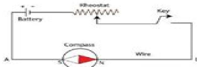
(a) When a key is open, the needle shows no deflection and it point in the N-S direction
