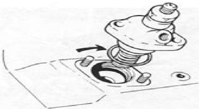
On later version engines an O-ring has been introduced as a seal between the injection pump and the block. Only so-called hard shims may be used on these engines when shimming. Hard shims are available in thicknesses of 0.2 mm (0.0079 in), 0.3 mm (0.0118 in), 0.6 mm (0.0024 in) and 0.9 mm (0.0354 in).
