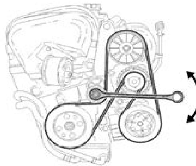
**Fig. 14: Removing/Installing Drive Belt**
