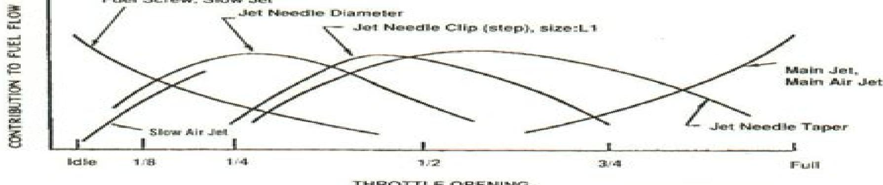
Each calibration part controls fuel flow at different throttle openings. The diagram above gives an idea which calibration part is the key at different throttle openings.
