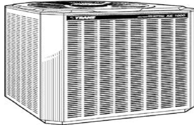
3. Avoid locating the unit where condensation and freezing of defrost vapor may annoy the customer. For instance, installing the unit under a bedroom, kitchen, or picture window may be annoying to the customer since condensate and fog will occur during the defrost cycle.
