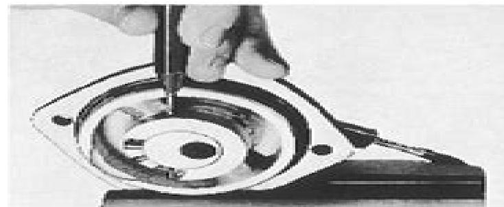
8. Knock out the load pin (1, figure above) and pull out the pin (2) and the eccentric piston (3). Remove the sealing ring (4). Wash the parts and check for wear. Replace parts if necessary.
