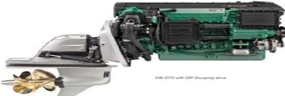
D6-370 with DP Drive propeller
